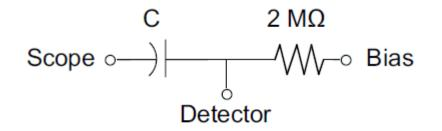
5. In the event that voltages >10% of the bias voltage are generated at the scope, the corrected voltage can be obtained from the following equation:
