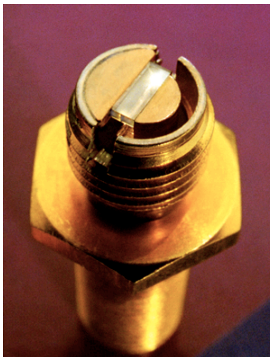
Figure 6: Photograph showing a diamond radiation detector. The diamond element is mounted within an SMA connector.
